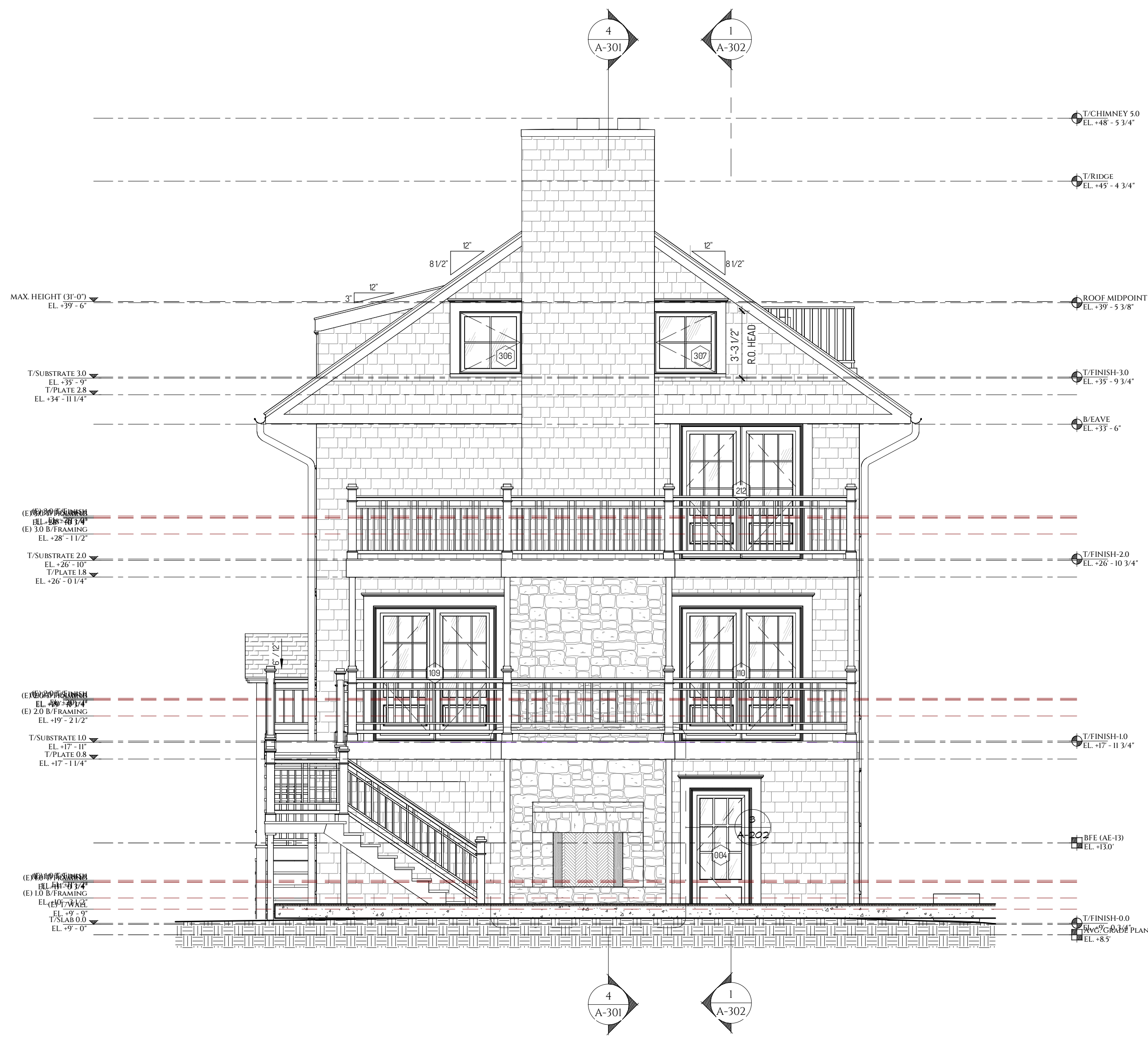
1 RIGHT (SOUTH / POOL) BUILDING ELEVATION A-202 SCALE: 1/4" = 1'-0"
