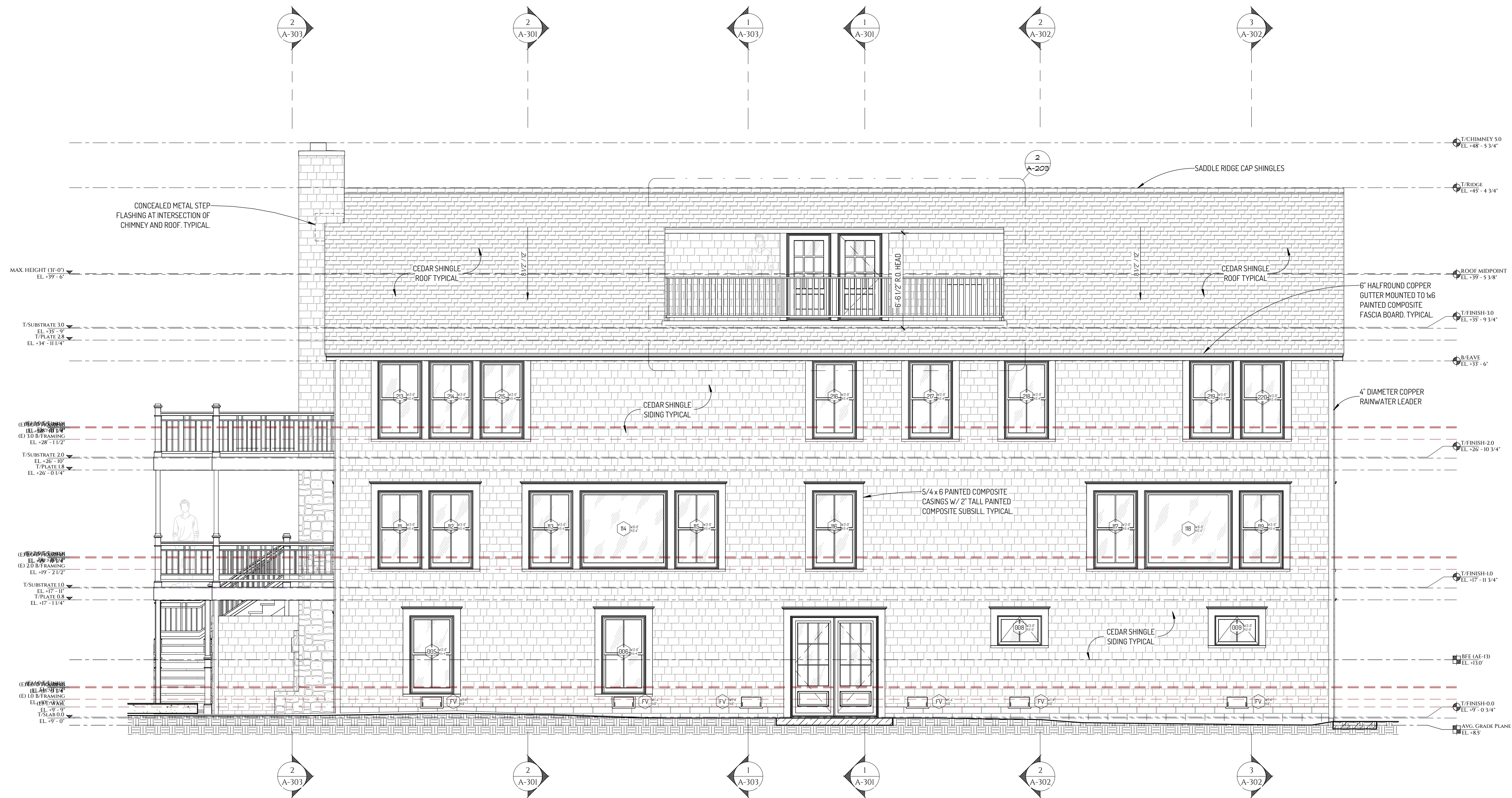
1 REAR (EAST / WATERFRONT) BUILDING ELEVATION SCALE: 1/4" = 1'-0"
