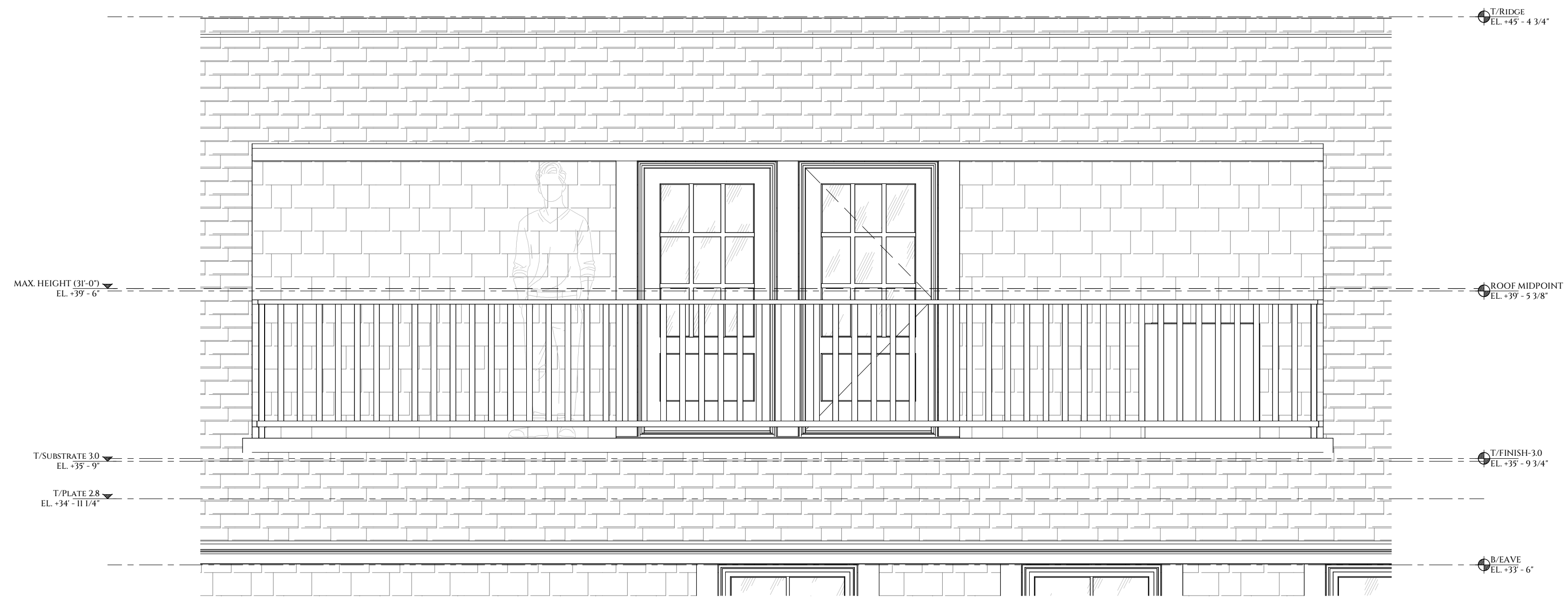
2 ROOF BALCONY REAR ELEVATION - CALLOUT SCALE: 1/2" = 1'-0"
