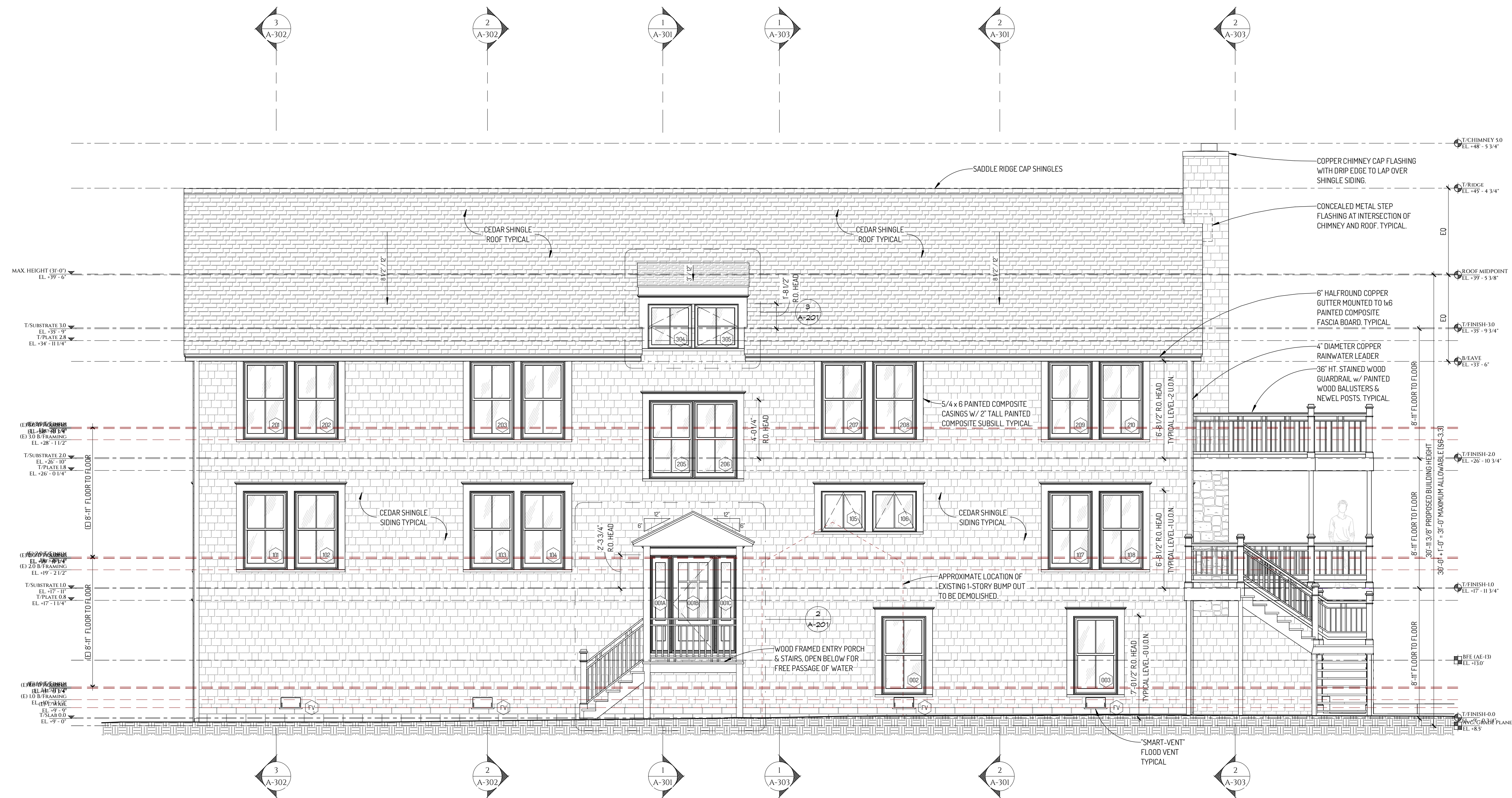
1 FRONT (WEST / STREET) BUILDING ELEVATION SCALE: 1/4" = 1'-0"
