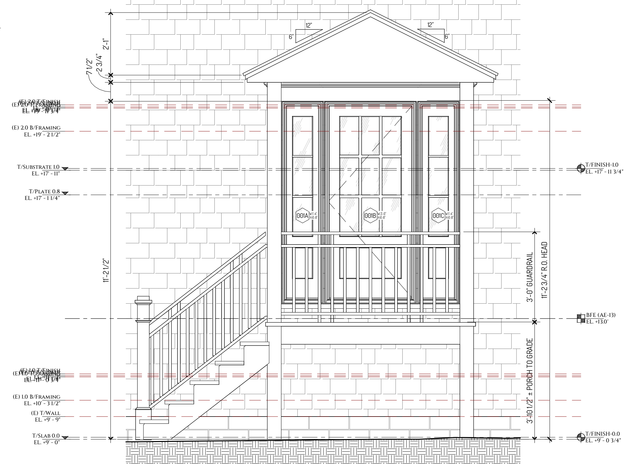
2 FRONT ENTRY ELEVATION - CALLOUT SCALE: 1/2" = 1'-0"
