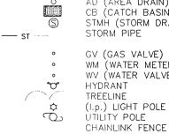
WM (WATER METER) WV (WATER VALVE) HYDRANT TREELINE (I.p.) LIGHT POLE UTILITY POLE CHAINLINK FENCE STOCKADE FENCE WIRE FENCE STONEWALL
