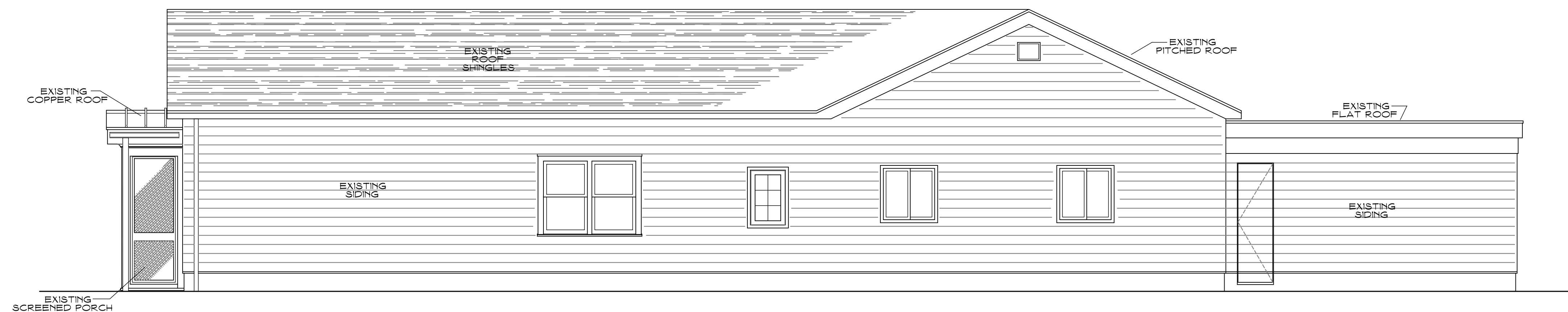
EXISTING EAST ELEVATION @ COTTAGE SCALE: 1/4"=1'-0"
