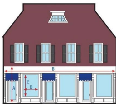
A: Height of Ground Floor C: Height of Glazing B: Width of Ground Floor D: Width of Glazing
