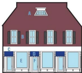
A: Decorative Window with Trim B: Two-over-two Windows, Shutters, Trim C: Sign Band, Trim D: Awnings E: Ground Floor Display Windows and Panels F: Inset Glazed Doors and Pilasters
