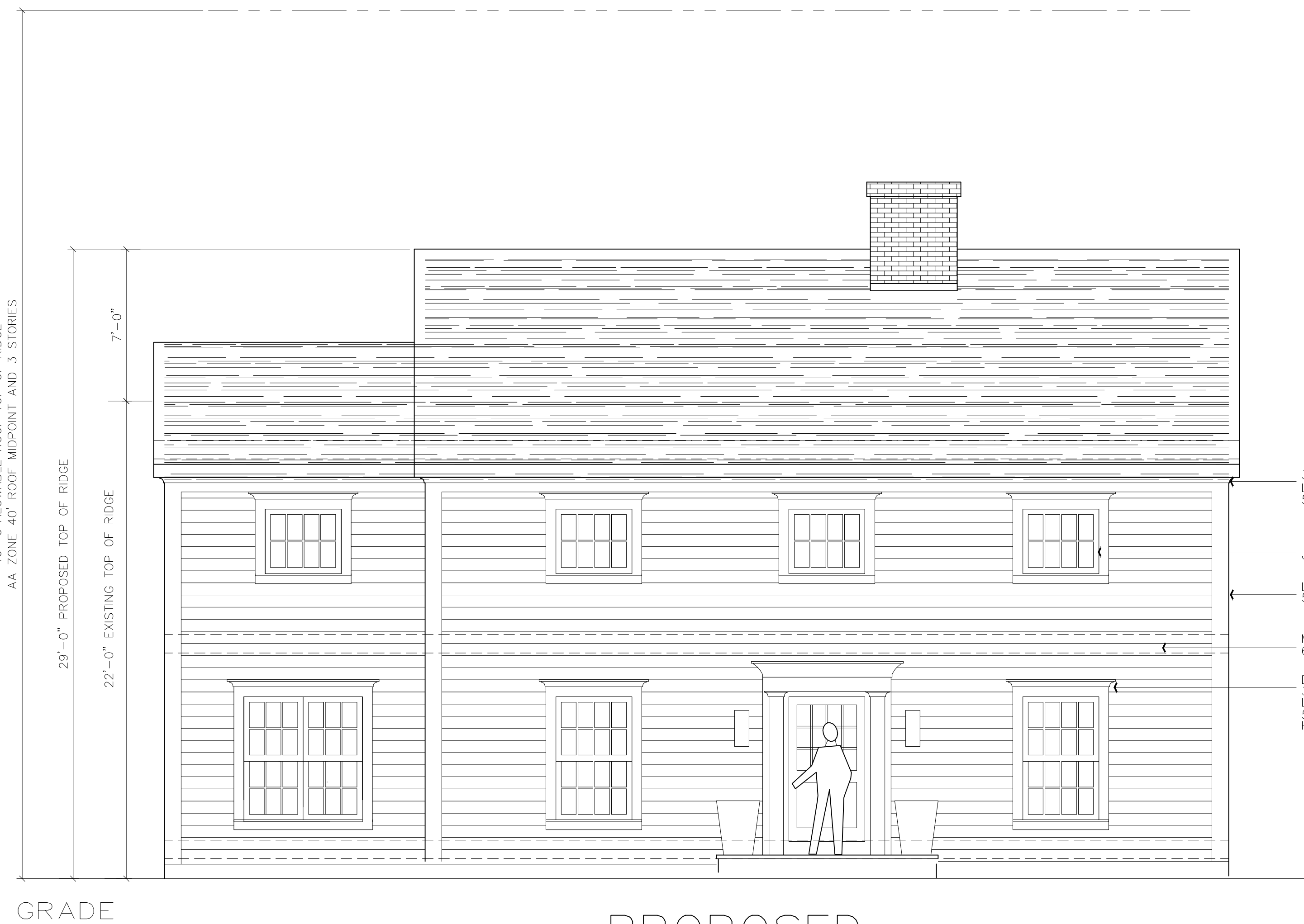
PROPOSED FRONT ELEVATION KINGS HIGHWAY NORTH
