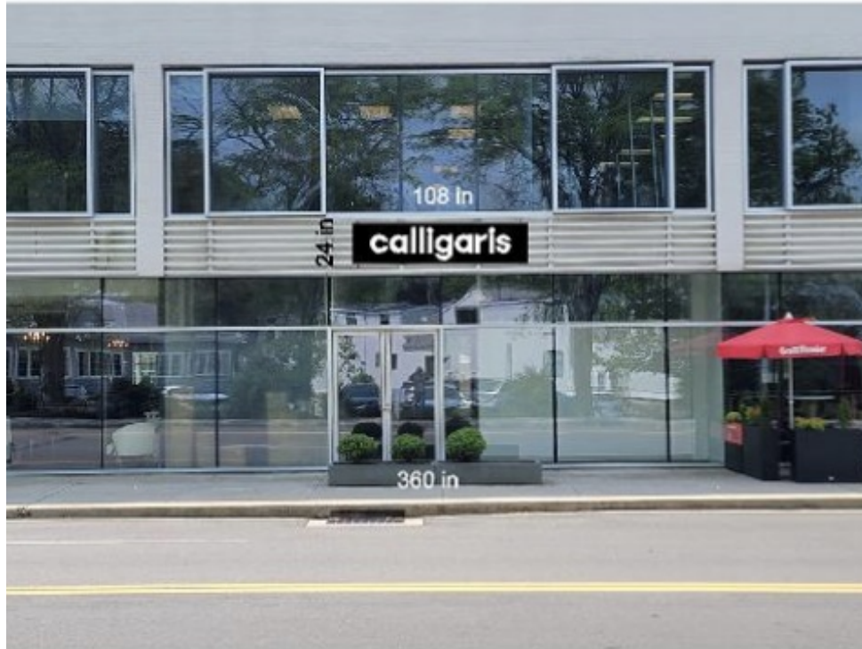
PROPOSED SIGN - FRONT OF BUILDING FRONT SIGN TO BE ILLUMINATED LETTERS (BACKLIT)
