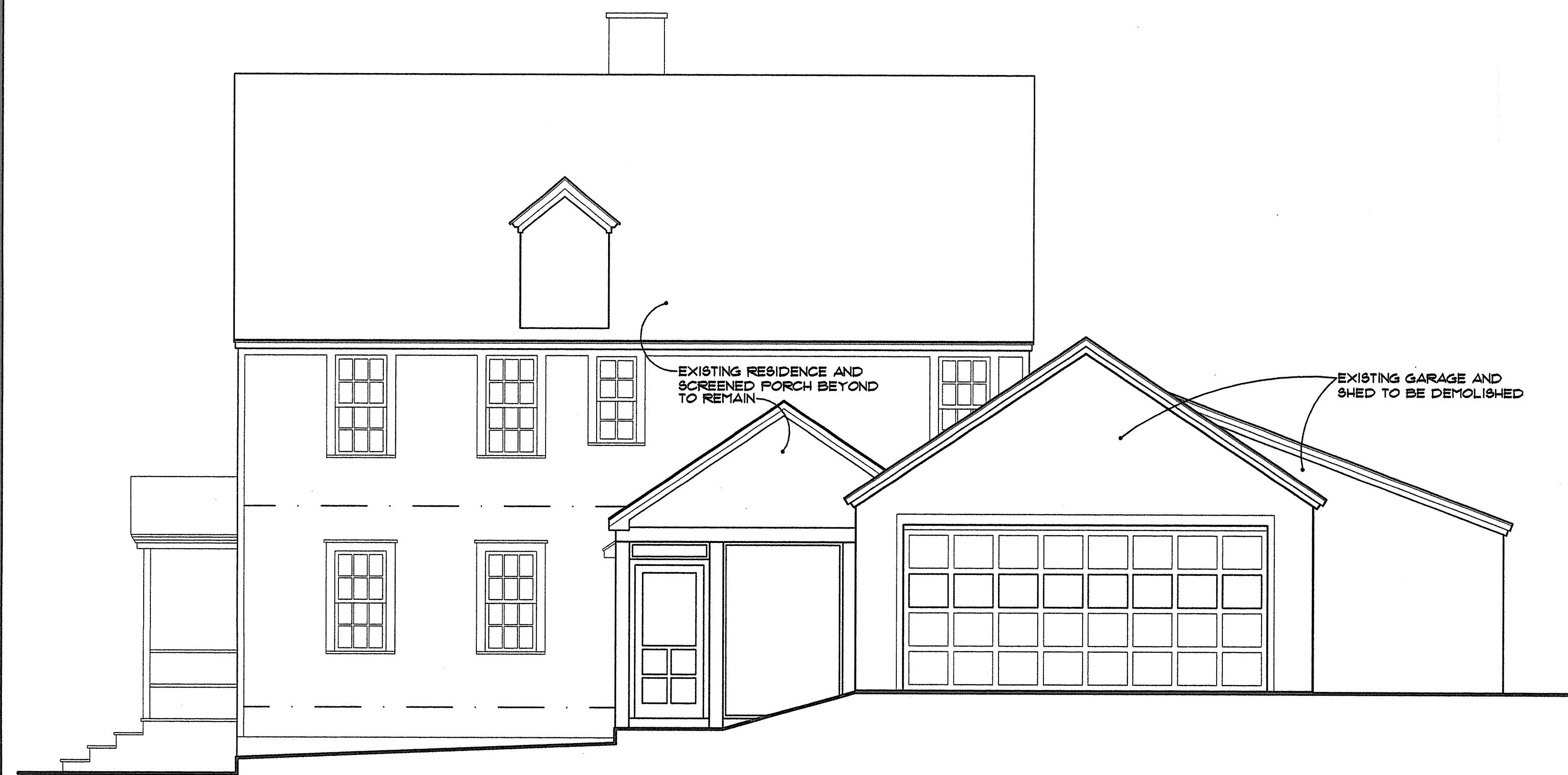
EXISTING NORTH ELEVATION DRIVEWAY ELEVATION
