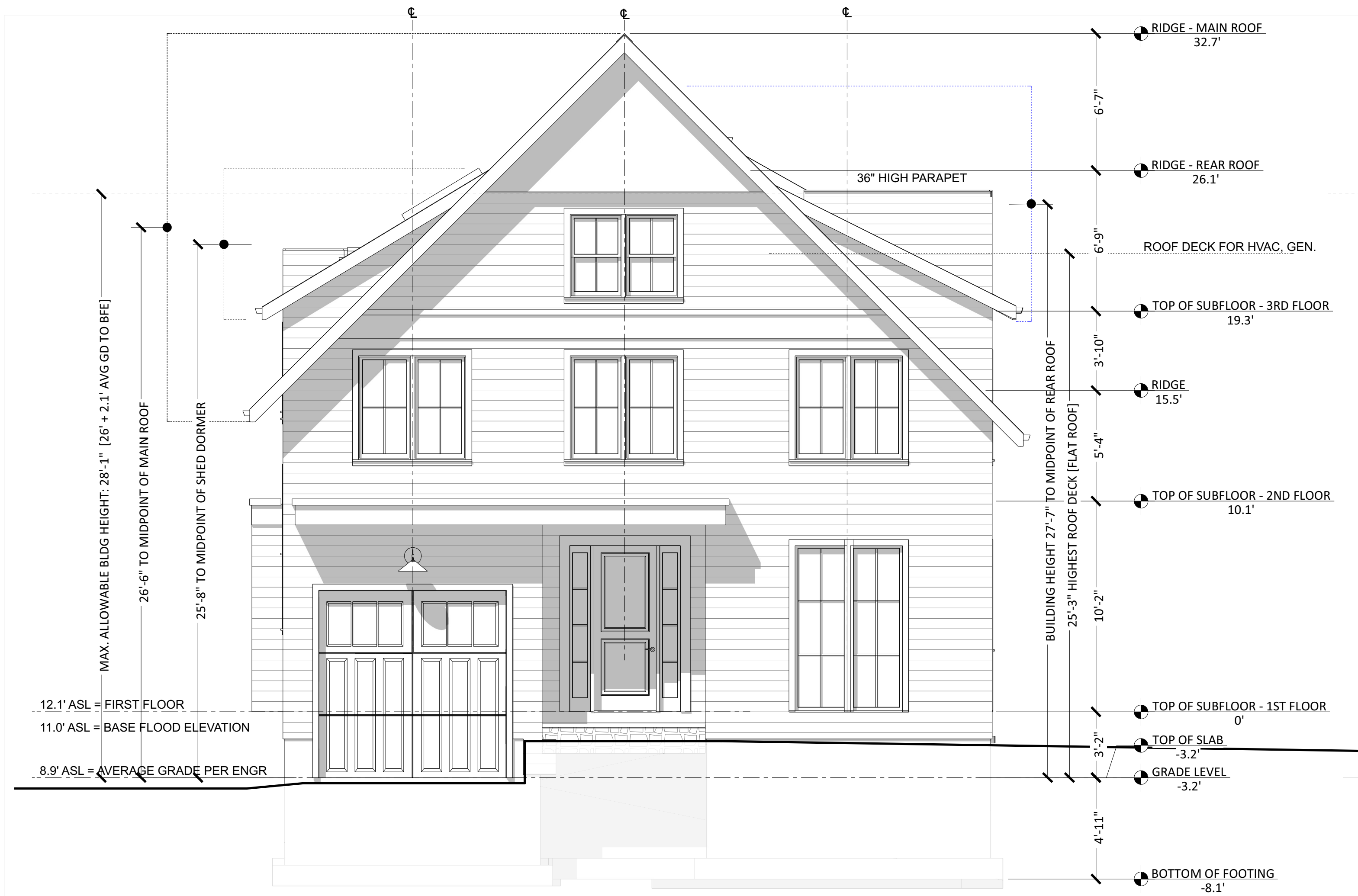
n. front [north] elevation 1/4" = 1'-0"
