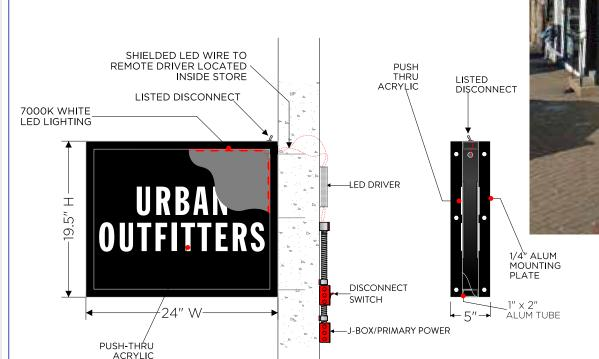
SIGN TO BE INSTALLED WITH BOTTOM OF SIGN ALIGNED WITH TOP OF WINDOW 11' - O" DISTANCE FROM GRADE TO B.O.S.
