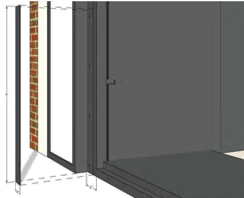
PROPOSAL FOR COVER TO CONCEAL JAMB ATTACHMENT POINTS
