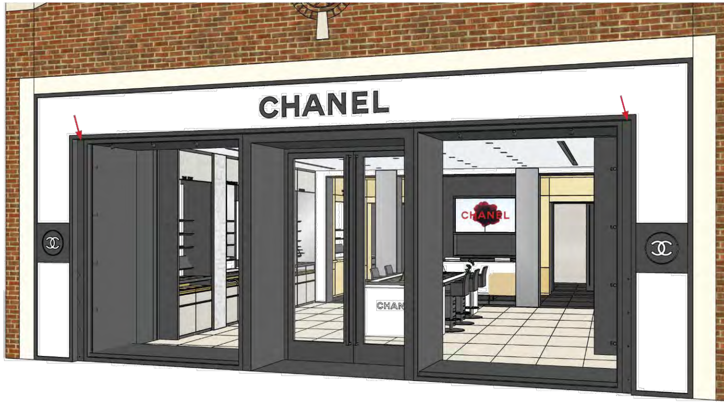
PROPOSED STOREFRONT - WITHOUT HYDRODEFENSE FLOOD PLANK (FP-530); ADDITION OF (2) 4" WIDE STRUCTURAL ELEMENTS
