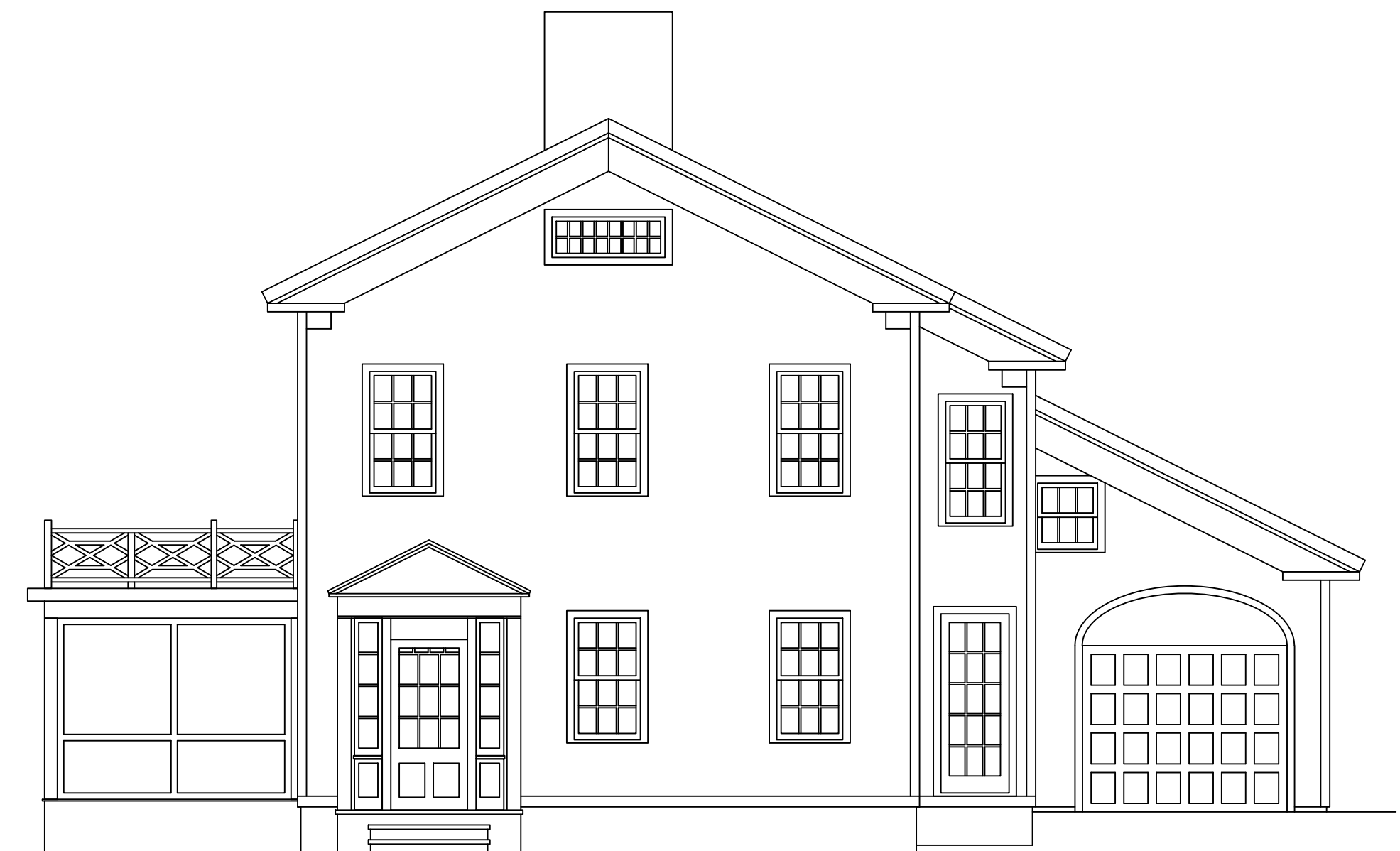
3 EXISTING FRONT ELEVATION 3/16"=1'-0"
