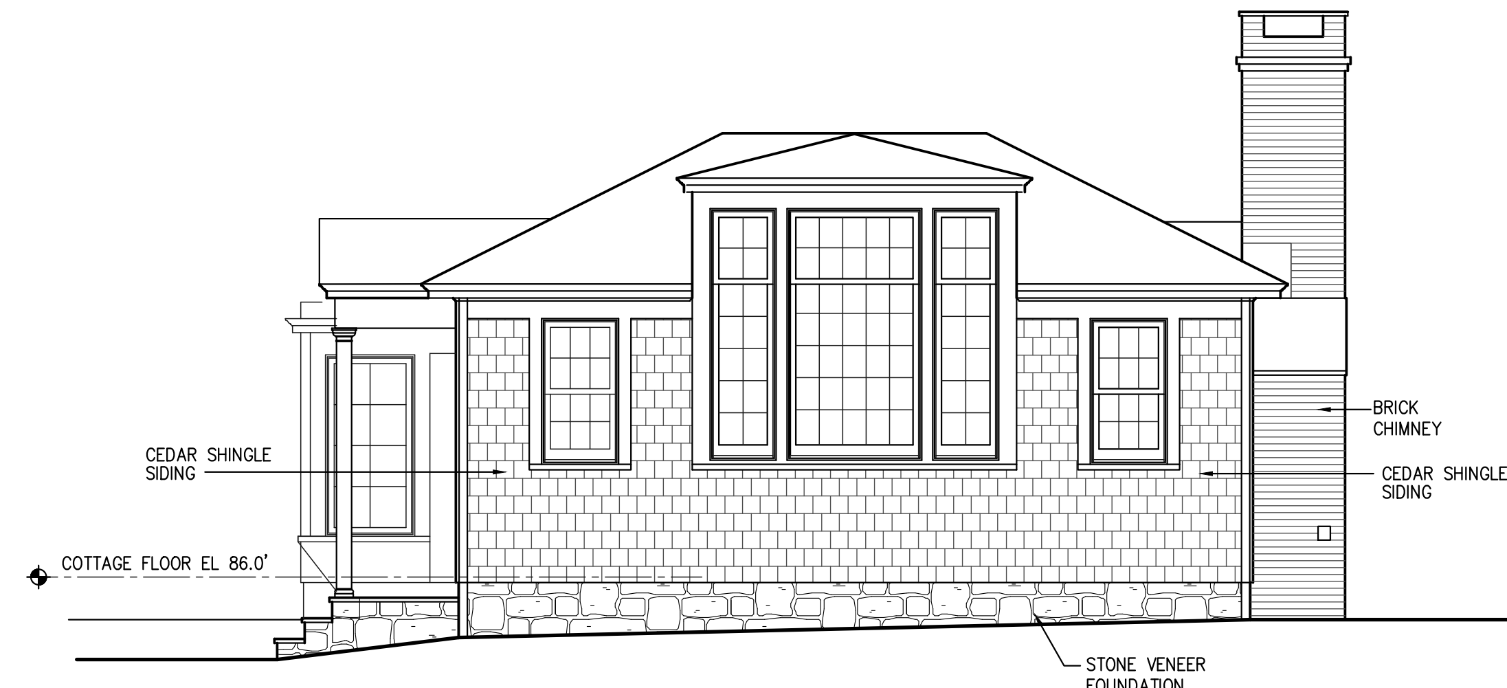
PROPOSED COTTAGE SIDE ELEVATION (NORTH) SCALE: 1/4"=1'-0"
