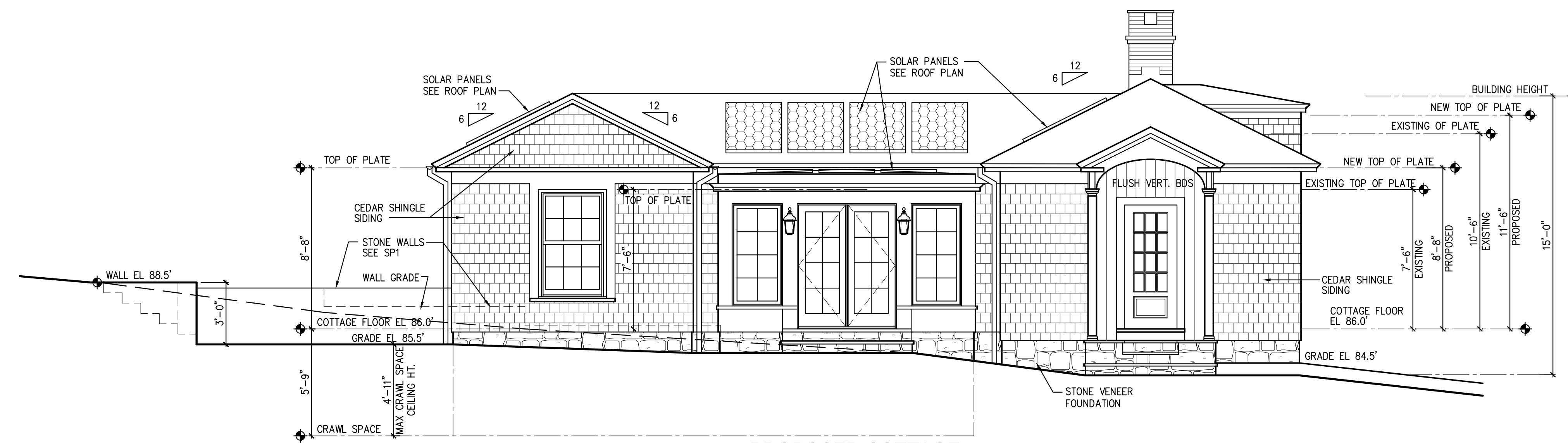
PROPOSED COTTAGE FRONT ELEVATION (EAST) SCALE: 1/4"=1'-0"
