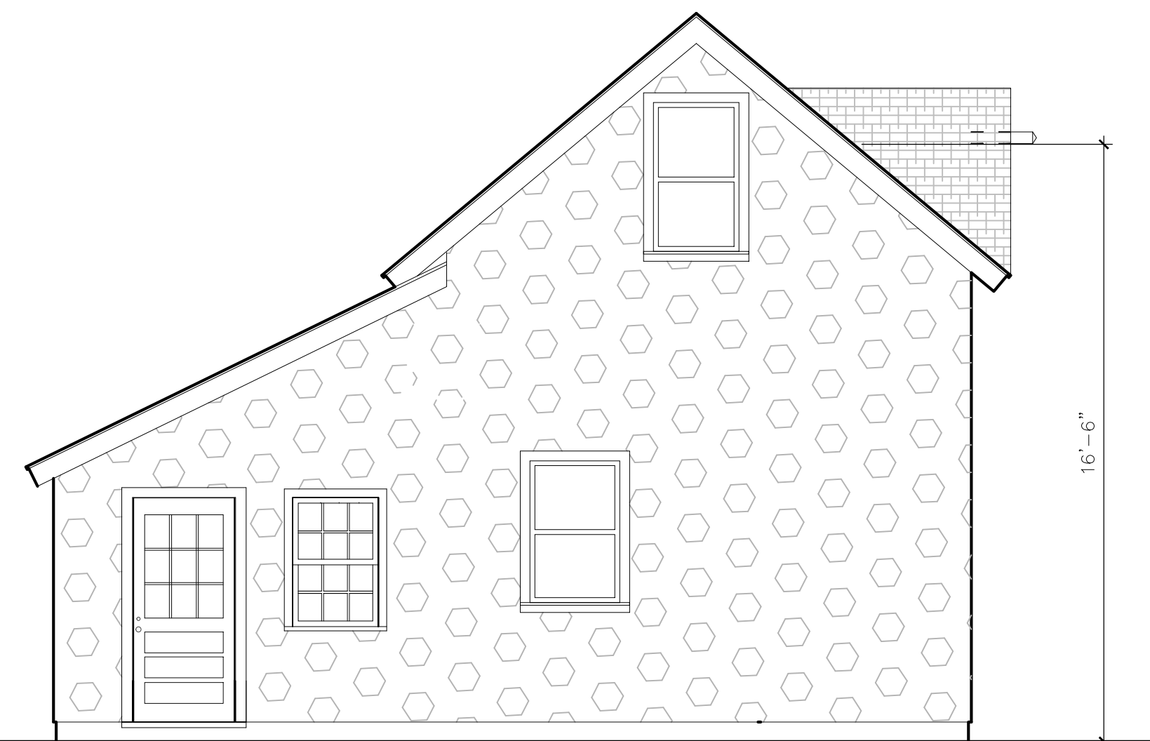
1 EXISTING WEST ELEVATION EX2 SCALE: 1/4"=1'-0"
