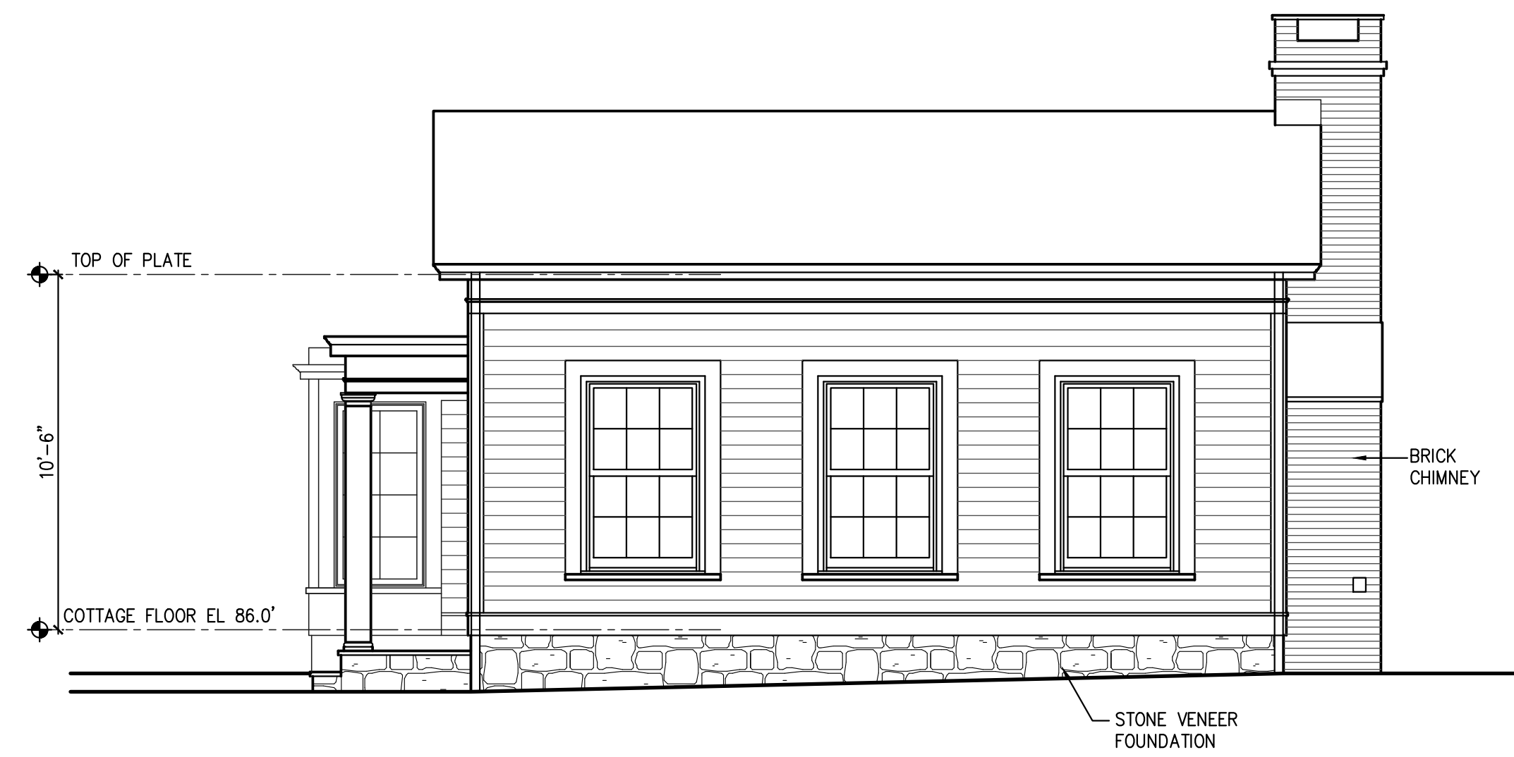
PROPOSED COTTAGE SIDE ELEVATION (NORTH) SCALE: 1/4"=1'-0"
