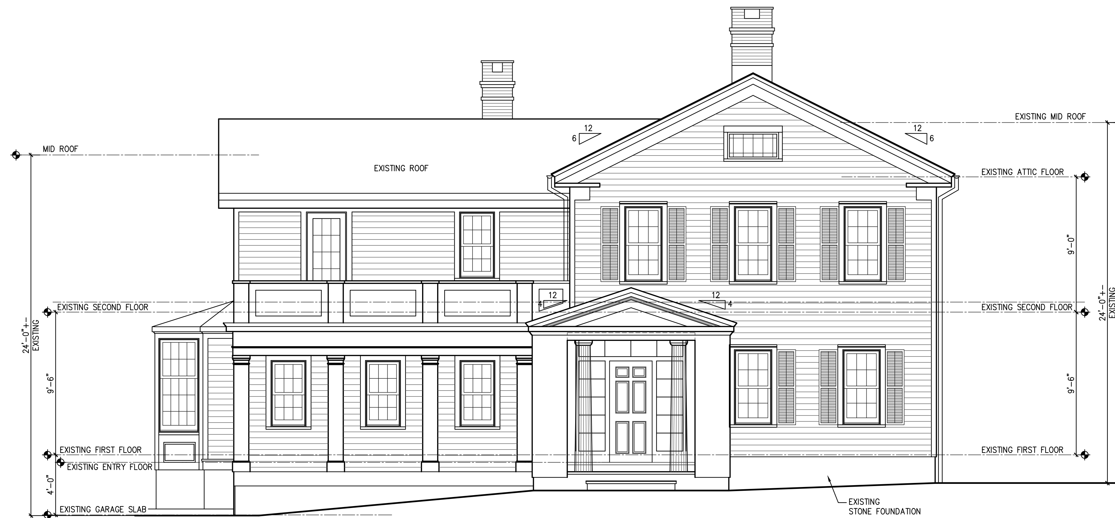
FRONT ELEVATION - WRIGHT STREET (NORTH) SCALE: 1/4"=1'-0"
