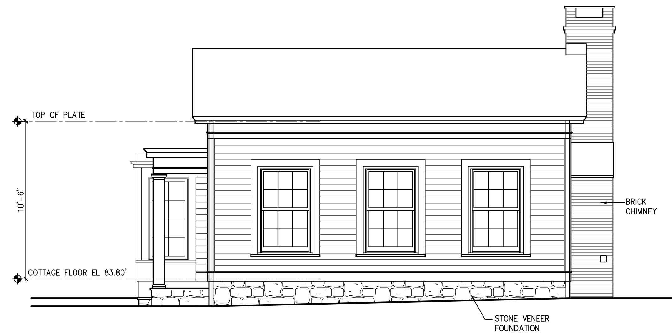
PROPOSED COTTAGE SIDE ELEVATION (NORTH) SCALE: 1/4"=1'-0"
