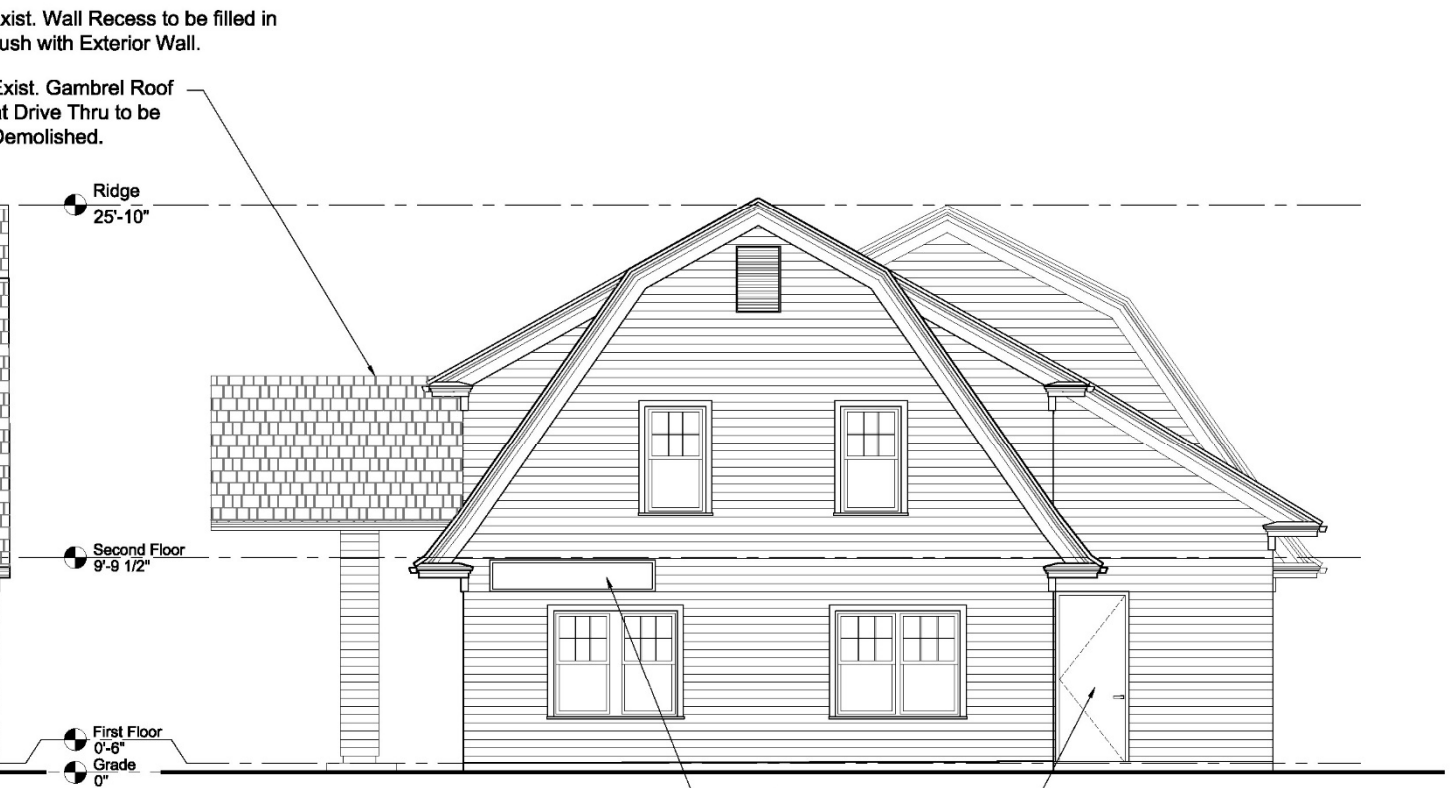
6 EXISTING EAST ELEVATION SCALE: 1/4" = 1'-0"
