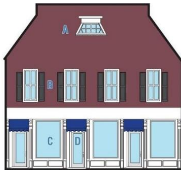
A: Decorative Window B: Typical Pattern for Second Story C: Ground Floor Display Windows D: Inset Glazed Doors
